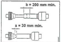
The P.T.O must be cut to a proper length, so it does not "bottom out" and bind. Remove the PTO to perform this operation. If the PTO is not cut to the proper length, it may cause damage to the PTO, gearboxes etc. See illustration for proper measurements.
