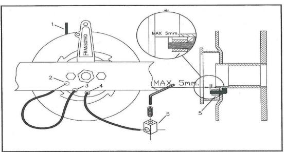
Drawing "B" Attaching cable to wire drum
